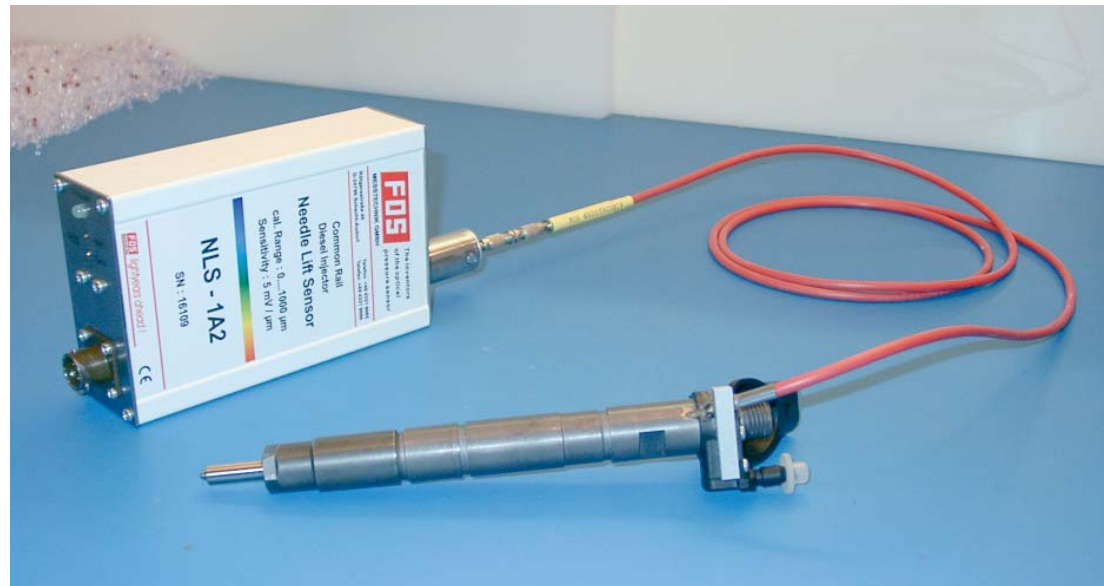
CR-Injector with fiberoptical needle lift measuring system
